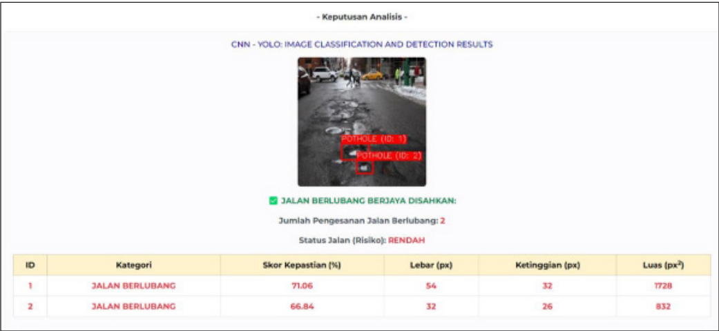
Figure 8. Detection results for uploaded road image showing pothole area
